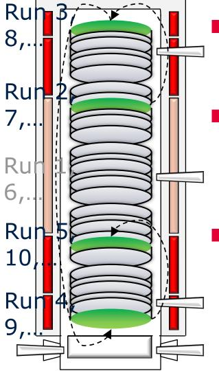
Zone 1,2,4 and 5 are cyclically measured by one (test) wafer run (interferometry or ellipsometry)
