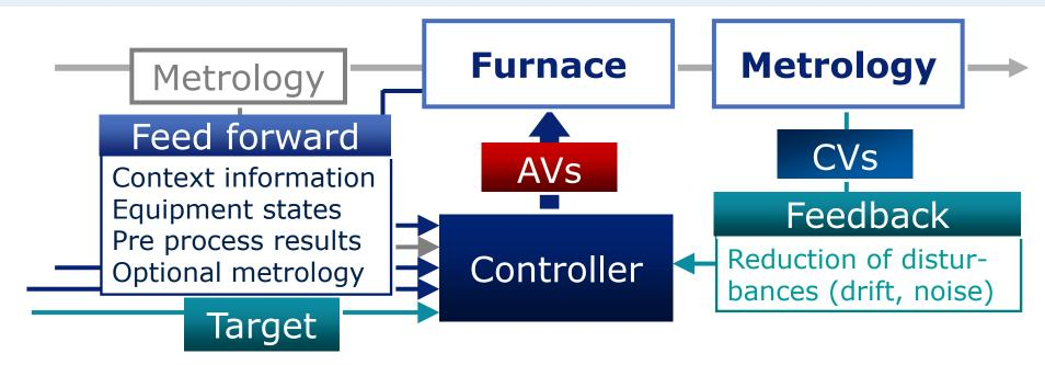
Actuating variables (AVs) are the process time (t), the temperatures  $(T_i)$  of 5 heating zones, the silane  $(F_{(SiH4)})$  and the dopant  $(F_{(Ph3)i})$  gas flows of 3 inlet zones
