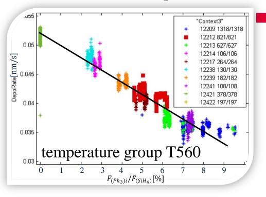
Deposition rate depends on dopant and silane gas flow relation. Deposition inhibitor gradient  $g_{F(rel)_3}$ was estimated as -0.12 nm/min/%
