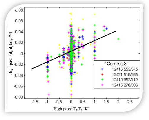
Temperature adjustments have an impact on relative deposition rate and thickness of 2 %/K (control gain  $g_{drT}$ )
