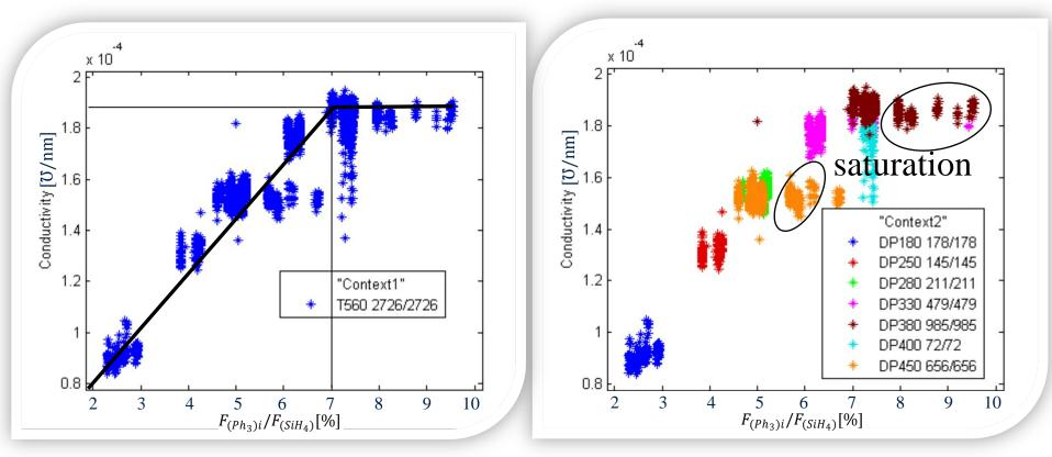
Conductivity gradient  $g_{\sigma}$  was estimated at 2.5e<sup>-3</sup>  $\Im/nm/\%$ for relative gas flow < 7 % within context group T560
